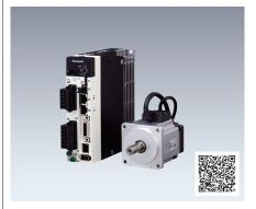
MINAS-A6series, rated output: 50W to 5kW. 3.2kHz frequency response. two-degree-of-freedom control system and fit-gain tuning featuring simple setup.
